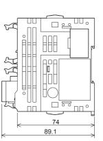
External color: Munsell 0.6B7.6/0.2 Unit: mm 35 mm width DIN rail can be installed
