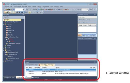
**6.** Set the converted program to "Scan". (In GX Works3 version 1.025B or later, the converted program is set to "Scan".) The converted program is stored in "No Execution Type". Set to scan by any of the following methods.
